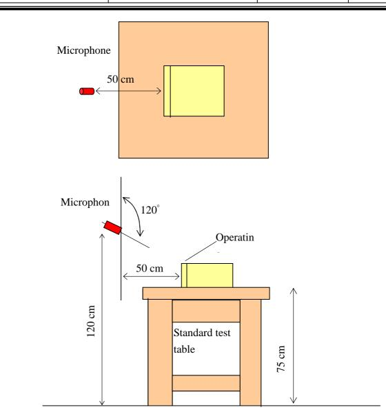
4-4. For B phase test, we determine the fan RPM to meet Shuttle acoustic SPEC in front side sound pressure (Idle & 3DMark 200x < =28 dBA).
